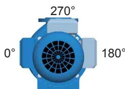
The terminal box alignment in a standard configuration is to the left (0°) when looking at the motor fan.
