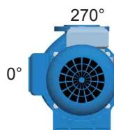
The terminal box alignment in a standard configuration is to the left (0°) when looking at the motor fan.
